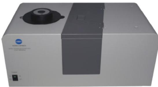
Slika 11. CM-3500d kolorimetar (Konica – Minolta, Japan)
