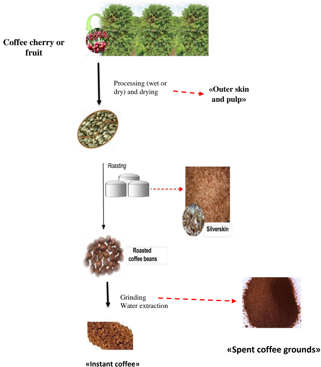
Figure 3. Coffee processing scheme (Mussato et al., 2011)
