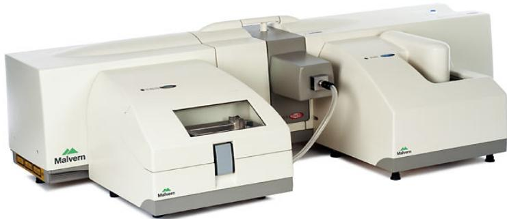
Slika 11. „Malvern Mastersizer 2000“ s vanjskom jedinicom Hydro 2000S (Malvern Panalytical, 2018)
