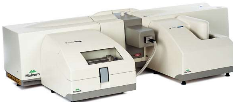
Slika 12. „Malvern Mastersizer 2000“ s vanjskom jedinicom Hydro 2000S (Malvern Panalytical, 2018)
