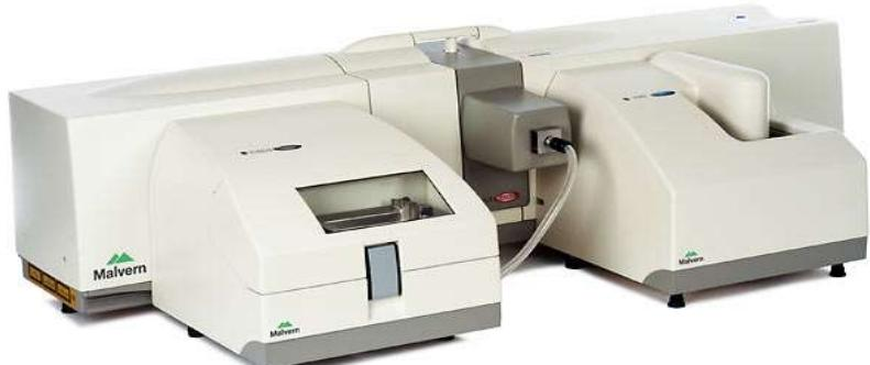
Slika 12. „Malvern Mastersizer 2000“ s vanjskom jedinicom Hydro 2000S (Malvern Panalytical, 2018)
