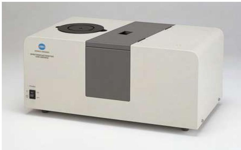
Slika 9. Kolorimetar KONICA-MINOLTA CM-3500-d, Japan (Konica Minolta, 2018)
