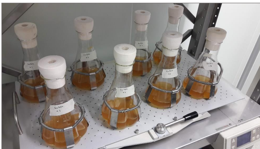
Figure 17. Production of AnGOX and GcGDH in shaking flasks
