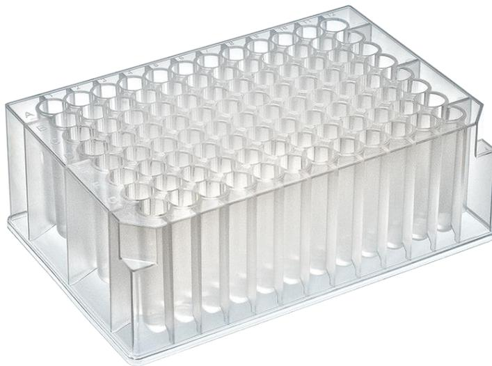
**Figure 4.** 96-deep well plate (adapted from Stellar Scientific)
