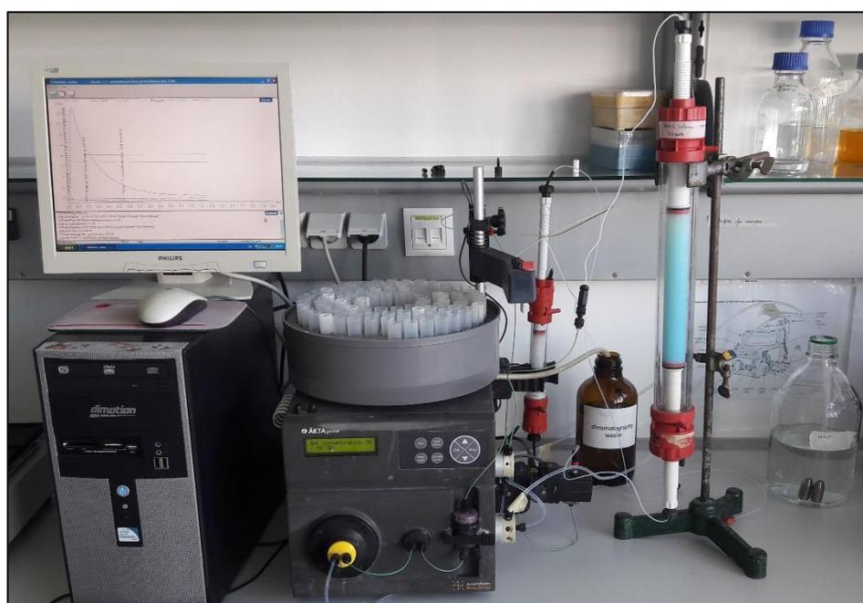
**Figure 6.** Äkta Prime system with IMAC column
