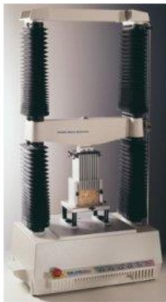
**Slika 5.** Analizator tekture TA.HDplus (Stable Micro Systems Ltd, 2009).
