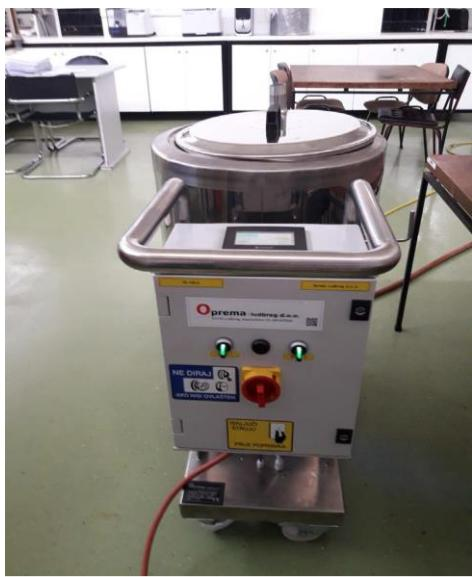
**Slika 6.** Šaržni pasterizator PS-100 (Burcar, 2019)
