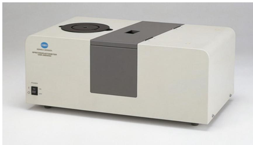
Slika 10. Kolorimetar Konica – Minolta CM-3500-d, Japan (Konica Minolta, 2020)
