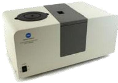
Slika 6. Kolorimetar KONICA-MINOLTA CM-3500-d, Japan
