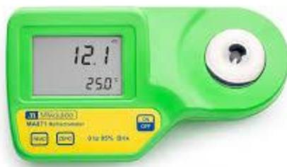
Slika 7. Digitalni refraktometar Milwaukee Instruments MA871 (Anonymous 5)
