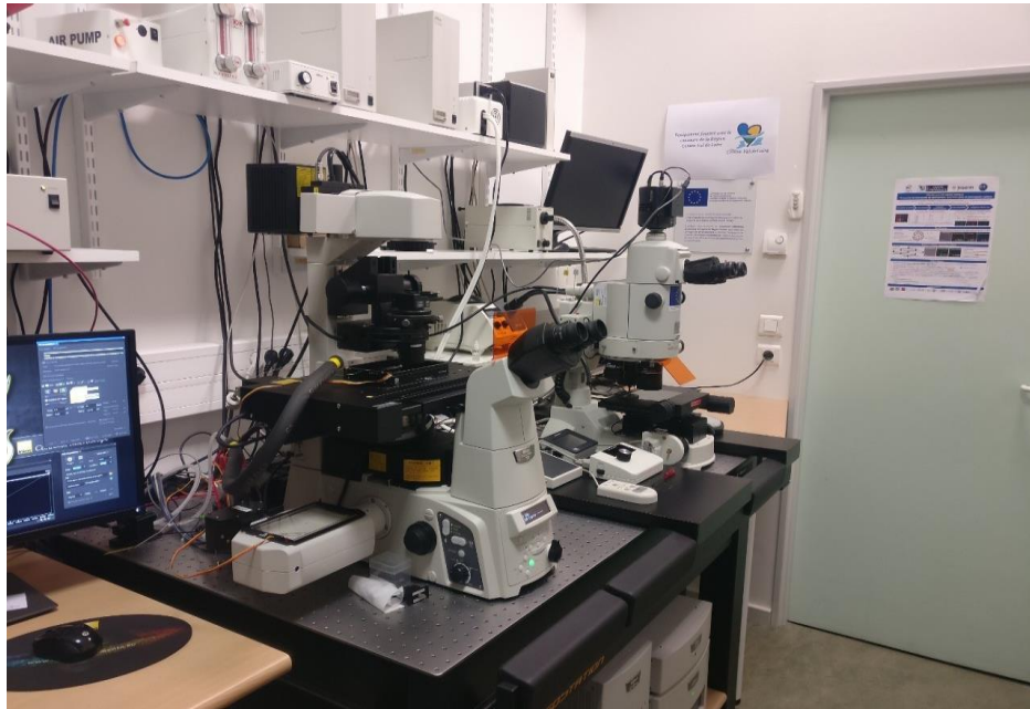
Figure 8. Microscopy equipment that was used - Nikon Eclipse Ti fluorescence inverted microscope equipped with a Photometrics EMCCD Evolve 512 camera and acquired with NIS-Elements software
