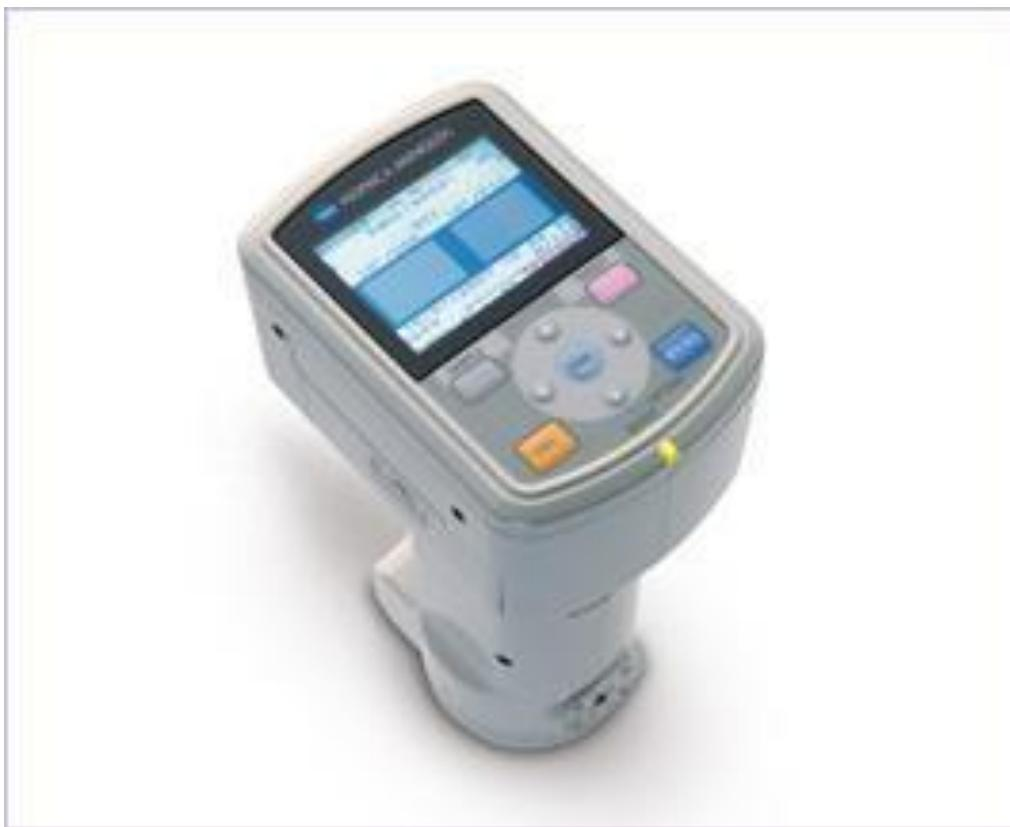
Slika 5. Spektrofotometar Konica Minolta CM-700d/600d (Anonymous 2, 2016)
