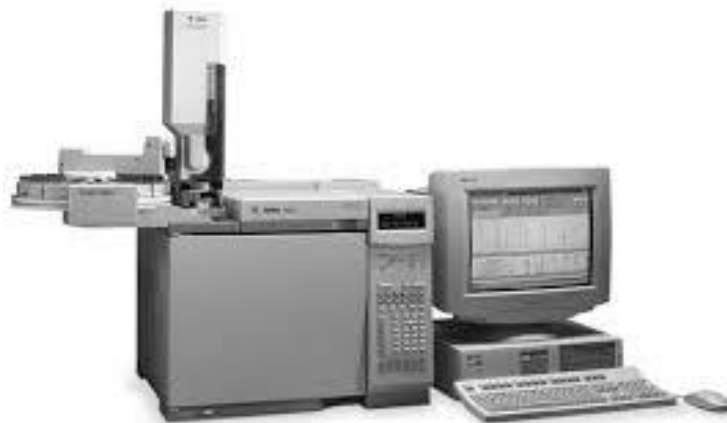
Slika 8. Plinski kromatograf Agilent Technologies 6890N - Network GC System (Anonymous 5).
