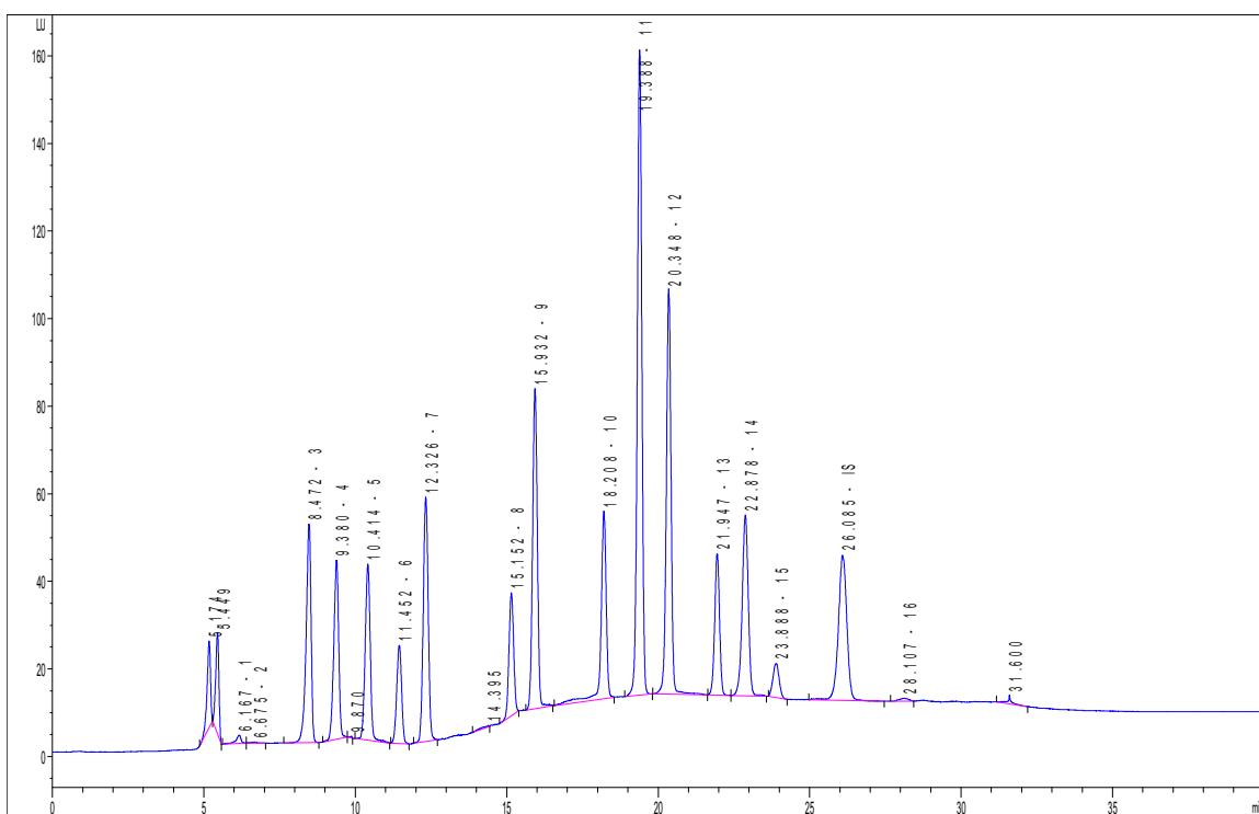
**Slika 48.** Kromatogram određivanja policikličkih ugljikovodika: (1) naftalen, (2) acenaftalen, (3) fluoren, (4) fenatren, (5) atracen, (6) flouranten, (7) piren, (8) benzo(a)atracen, (9) krizen, (10) benz(b)fluoranten, (11) benz(k)fluoranten, (12) benz(a)piren, (13) dibenzo(a)atracen, (14) benzo(g,h,i)perilen, (15) indeno(1,2,3 cd)piren, (IS) bezno(b)krizen
