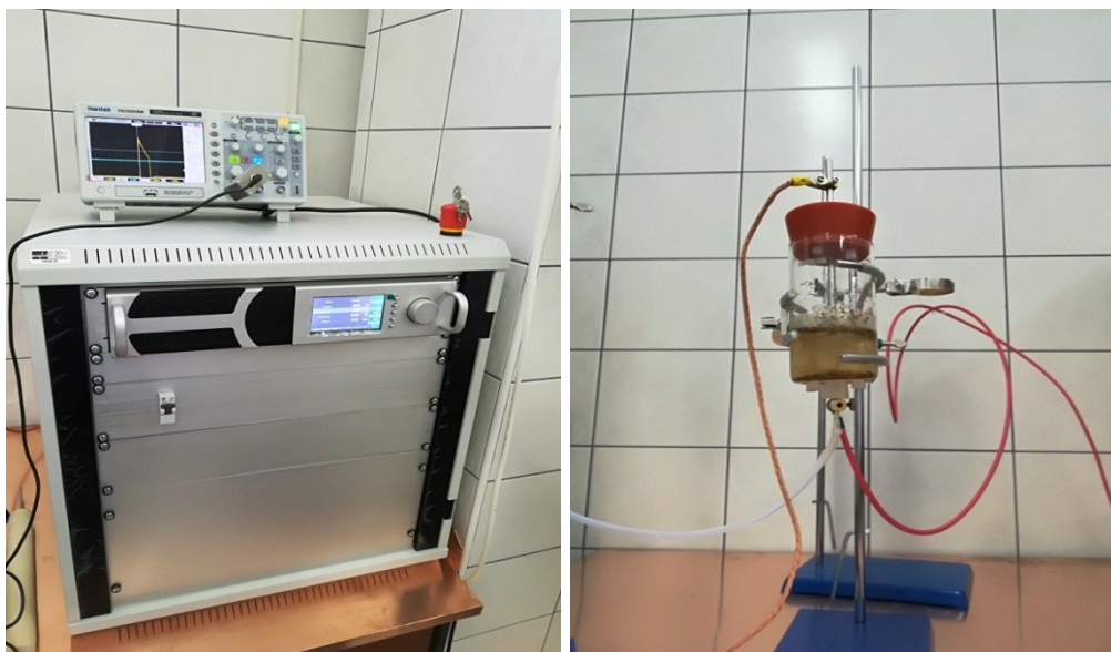
Slika 8. Plazma generator IMP-SSPG-1200 i reaktor (Anonymous, 2018)
