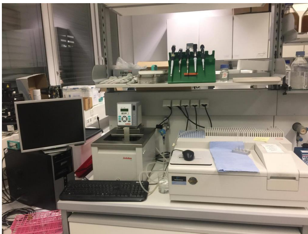
Figure 12. Spectrophotometer Lambda 35 with water bath.
