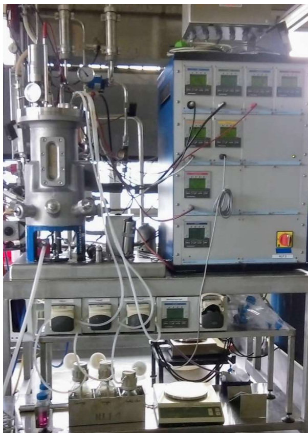
Figure 8. Bioreactor connected to control cabinet and acid/base/antifoam pumps
