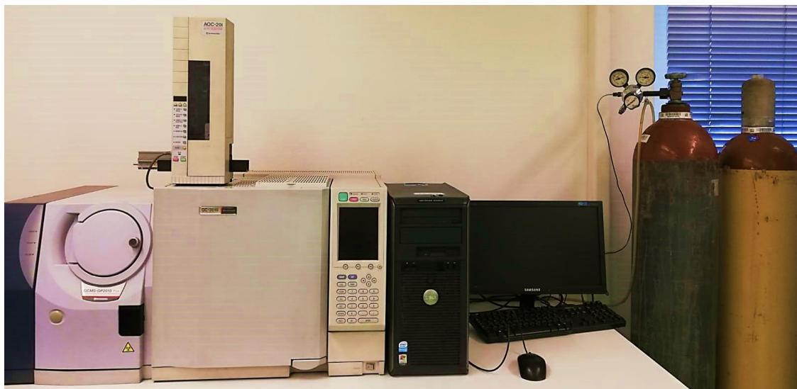
Slika 6. Plinski kromatograf s masenim spektofotometrom (GC-MS), Shimadzu QP2010PLUS, Japan.
