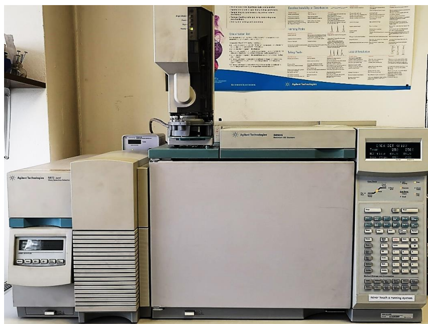
Slika 9. Plinski kromatograf Agilent Technologies 6890N Network GC System s masenim detektorom tipa 5973 inert Mass Selective Detector (Medved i Tonković, 2020)
