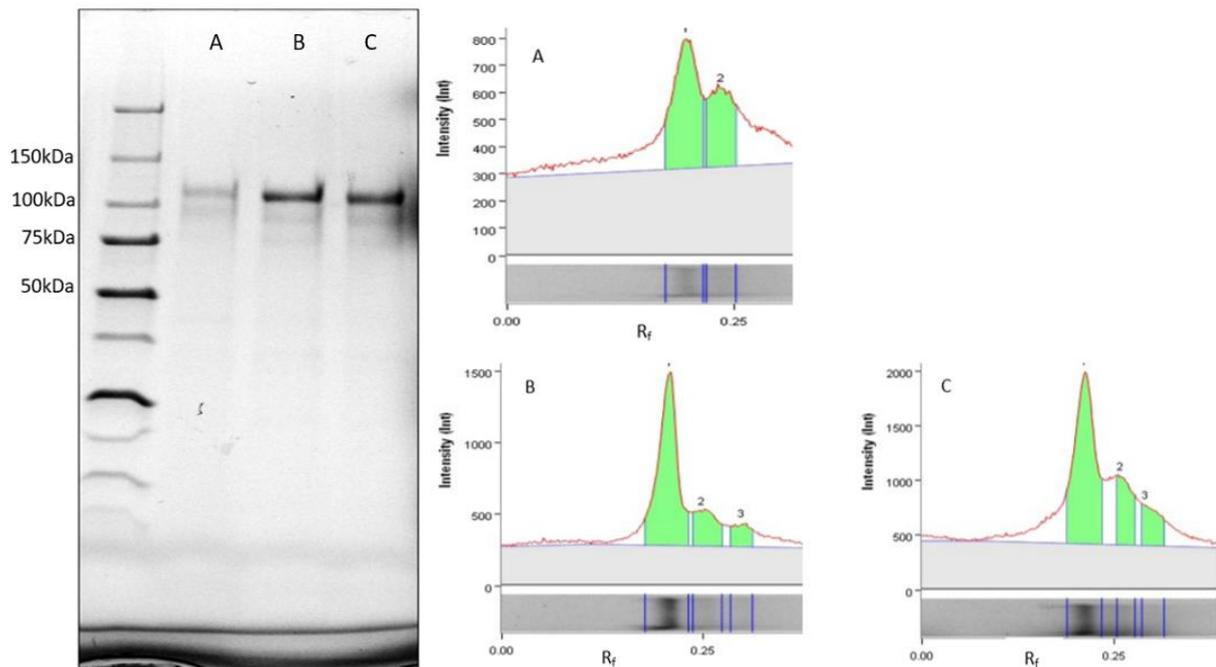
**Figure 22.** SDS-PAGE of HIC and AEX fractions (left) and lane and band analysis by Imager ChemiDoc™ XRS+ 5.2.1. Imager Software for AEX band (right). Bands analyzed: pooled HIC fractions (A), AEX fraction 15 (B) and AEX pooled fractions
