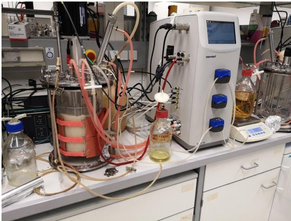
Figure 9. 5-L BioFlo fermenter with the Eppendorf BioFlo120 fermentation system as control process control system
