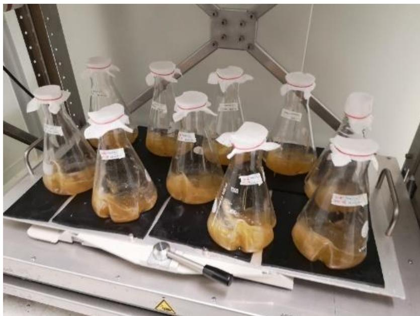
**Figure 15.** Production of *MtCDH* in shaking flasks
