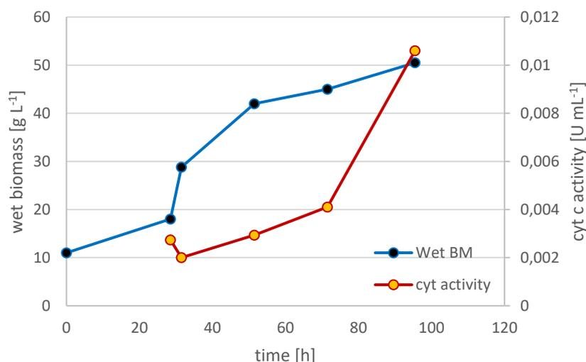
**Figure 19.** Production of the G317S *MtCDH* in shaking flasks with curves for wet biomass concentration and cytochrome *c* activity
