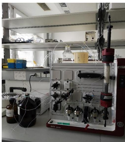
**Figure 11.** Äkta Puresystem with Q Source 30 column
