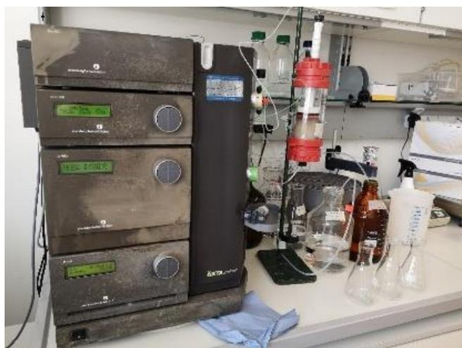
**Figure 10.** Äkta Explorer system with Phenyl Sepharose Fast Flow column
