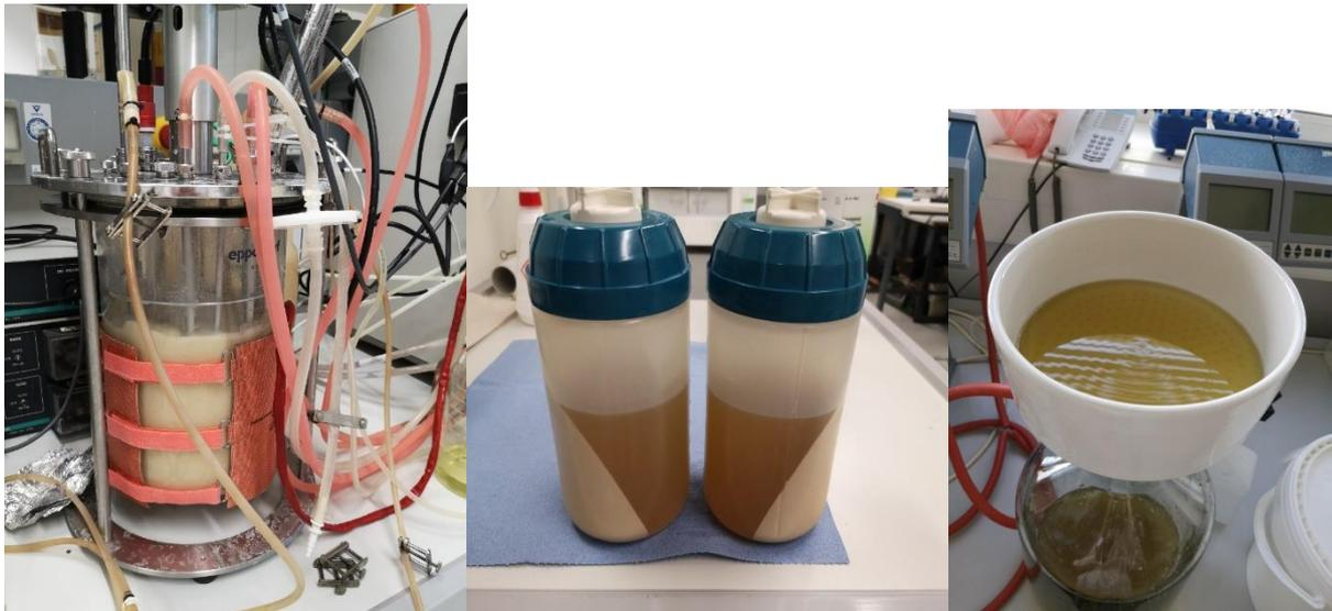
**Figure 27.** Fermentation in BioFlo bioreactor (left), medium after centrifugation (middle) and supernatant vacuum filtration (right)
