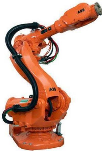
Slika 3. ABB IRB robot (Anonymous 3)
