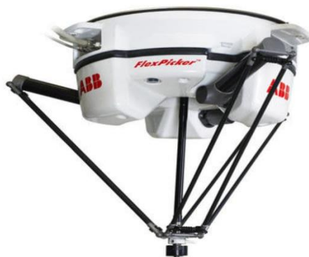
Slika 13. Flex picker robot (Anonymous 7)
