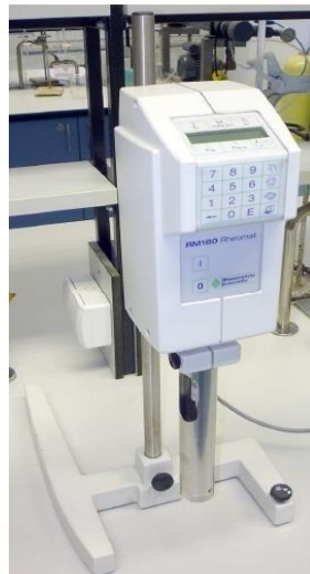
Slika 10. Rotacioni reometar Rheometric Viscometer (Model RM 180, Rheometric Scientific, Inc., Piscataway, USA)
