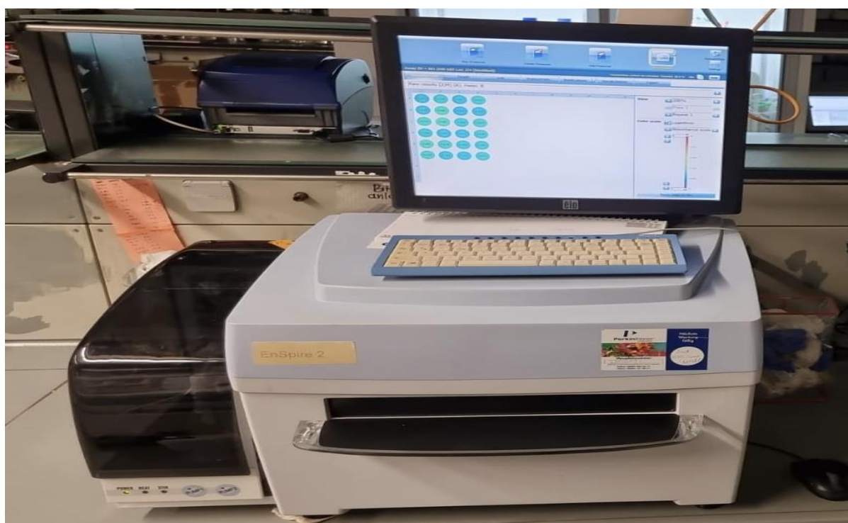
Figure 5. EnSpire Multimode Plate Reader (Perkin Elmer, Waltham, USA)
