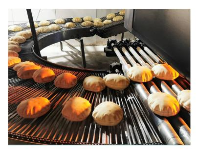
**Figure 3.** Jordan *Kmaj* in an automatic baking line. The inflation of bread due to the thermal expansion of the gases is clearly visible.
