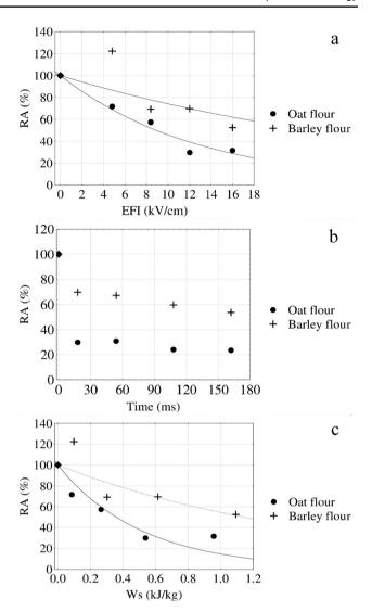
**Fig. 1** The residual activity (RA) of oat and barley flour β-glucanase exposed to **a** different EFI at constant treatment time (18 ms), **b** different treatment time (ms) at constant EFI (12 kV/cm), and **c** residual β-glucanase activity in oat and barley flour submitted at different specific energy inputs supplied by high-intensity pulsed electric fields from 4.8 to 16 kV/cm for 18 ms. The values are shown as mean  $\pm$  standard deviation (n=2)
