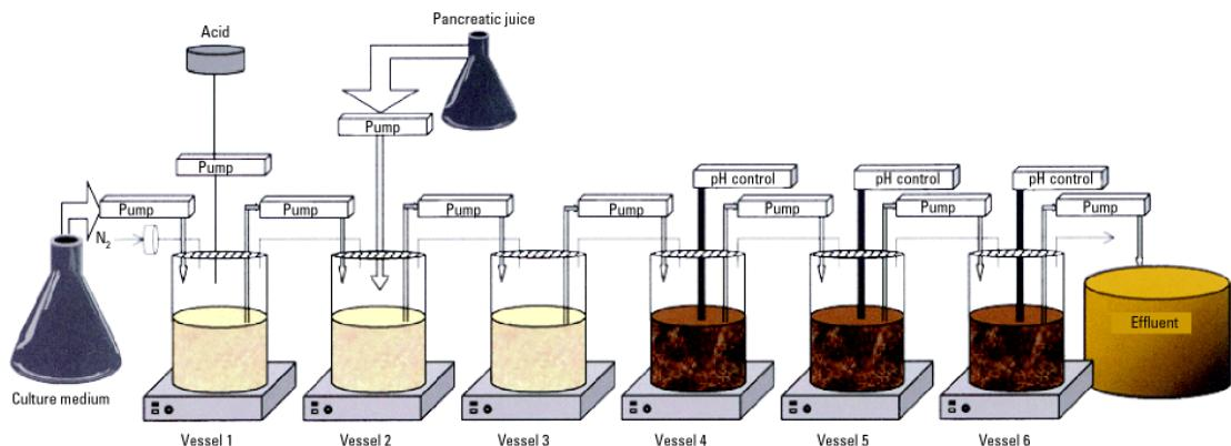
**Slika 5: Simulator for Human Intestinal Microbial Ecosystem (SHIME) model**
