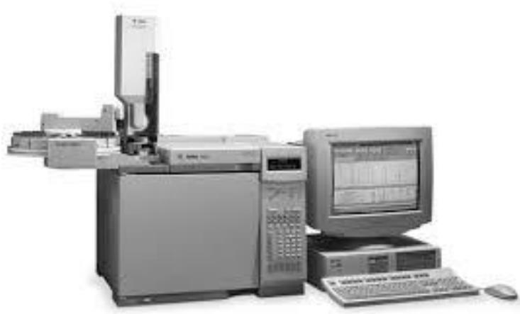
Slika 8. Plinski kromatograf Agilent Technologies 6890N - Network GC System
