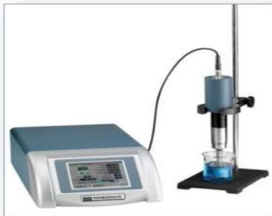
Slika 1: Ultrazvučni procesor model S-4000 (MisonixSonicators, Newtown, Connecticut, SAD)
