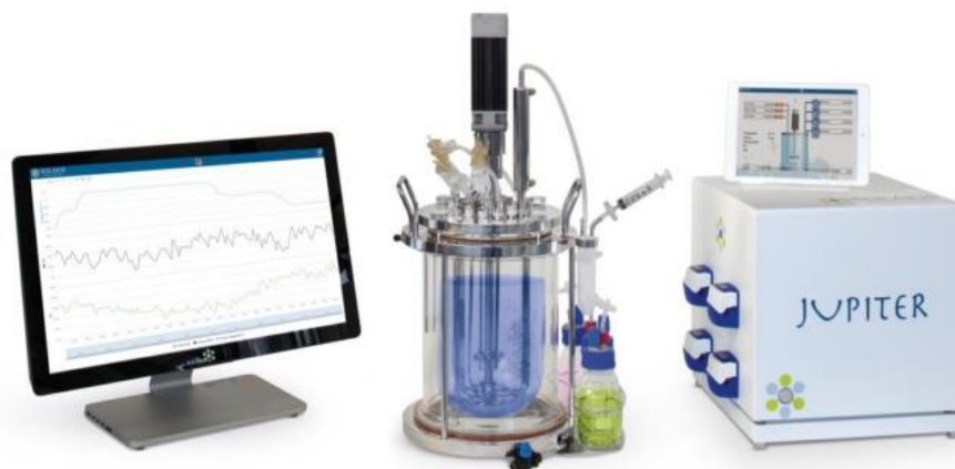
Slika 10. Bioreaktor Jupiter 2.0 (User and Maintenance manual for Jupiter 2.0., 2016)
