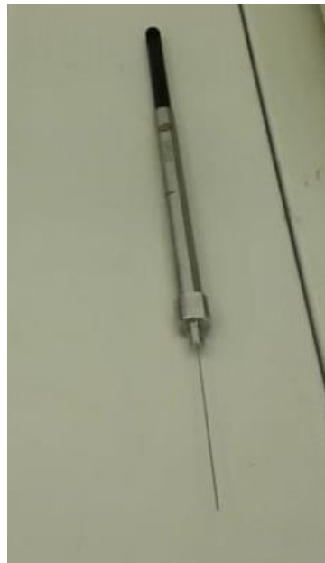
Figure 11. SPME fibre (own picture)
