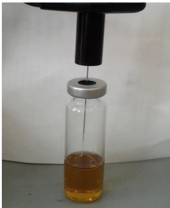
Figure 12. SPME sampling (own picture)
