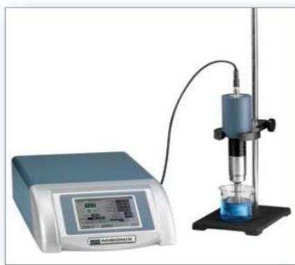
**Slika 3.** Ultrazvučni procesor model S-4000 (MisonixSonicators, Newtown, Connecticut, SAD)
