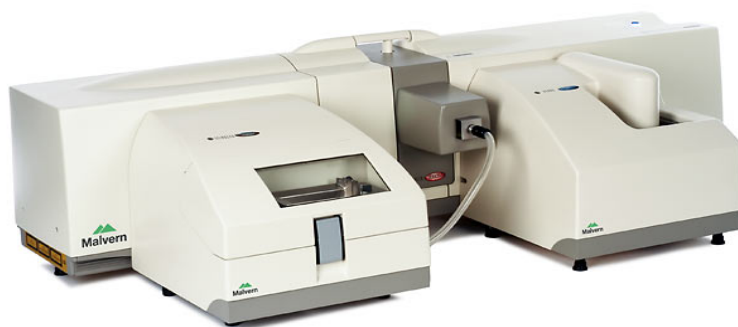
Slika 11. „Malvern Mastersizer 2000“ s vanjskom jedinicom Hydro 2000S (Malvern Panalytical, 2018)
