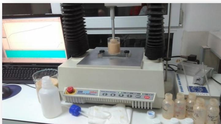
Slika 9. analizator tekture TA.HDPlus (Stable Mycro System, Engleska)
