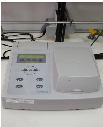
Slika 2. Spektrofotometar (Helios Epsilon, Thermo Fischer Scientific, Waltham, Massachusetts, SAD).
