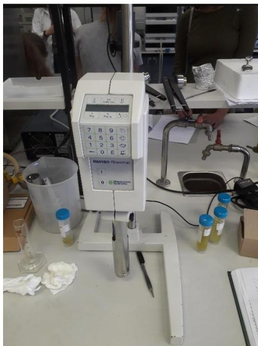
**Slika 4.** Reometar (RM 180, Rheometric Scientific, Inc., Piscataway, USA)
