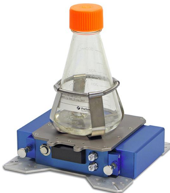
Figure 5. PreSens baffled flask that allows online monitoring of dissolved oxygen, biomass and pH (adapted from PreSens)
