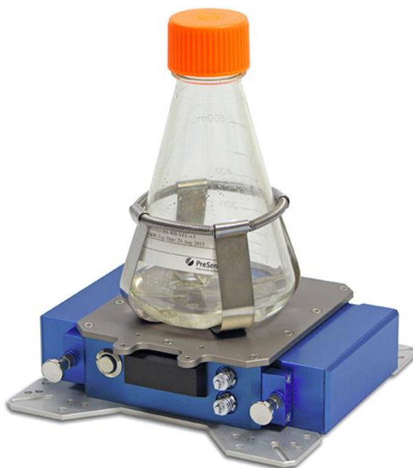
Figure 5. PreSens baffled flask that allows online monitoring of dissolved oxygen, biomass and pH (adapted from PreSens)
