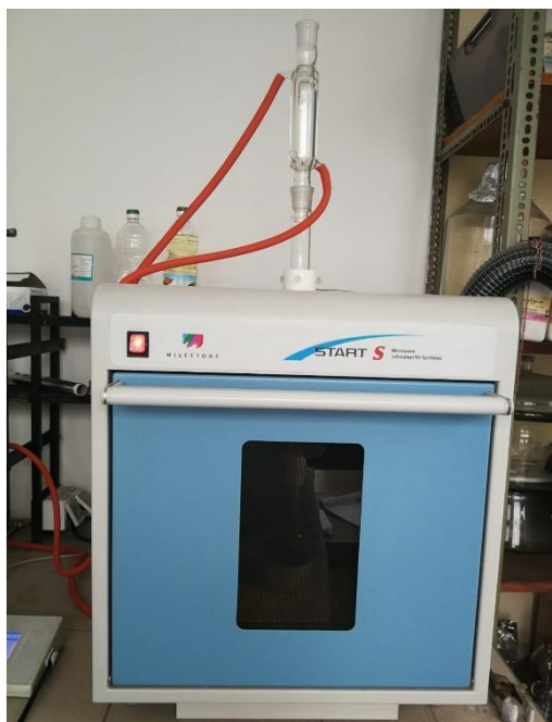
Slika 4. Mikrovalni reaktor, Start S Microwave Labstation for Synthesis (Milestone, Italija) (foto: Jurić, 2019)
