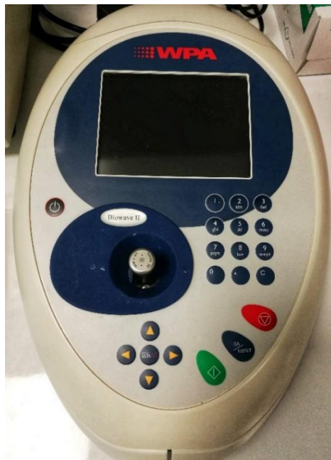
Figure 10. WPA Biowave II UV-Vis Spectrophotometer, Biochrom.
