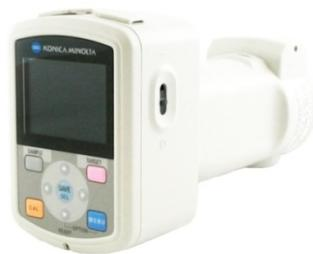
Slika 12. Spektrofotometar Konica Minolta (CM-700d, Minolta, Japan) (Anonymous 6, 2020)
