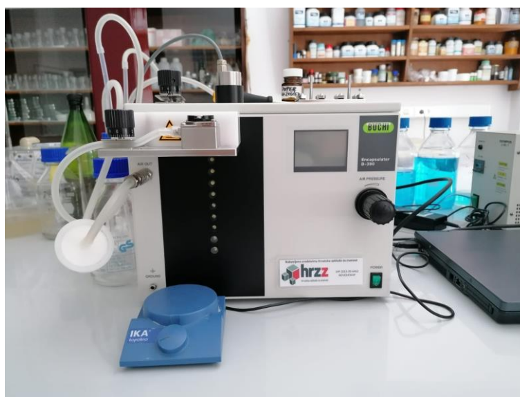
Slika 6. Inkapsulator (Büchi Encapsulator B-390)
