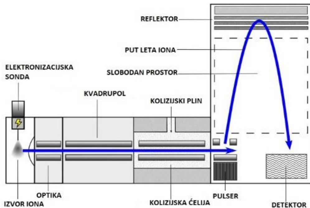
**Slika 9.** Shematski dijagram Q-TOF uređaja (Allen i McWhinney, 2019)
