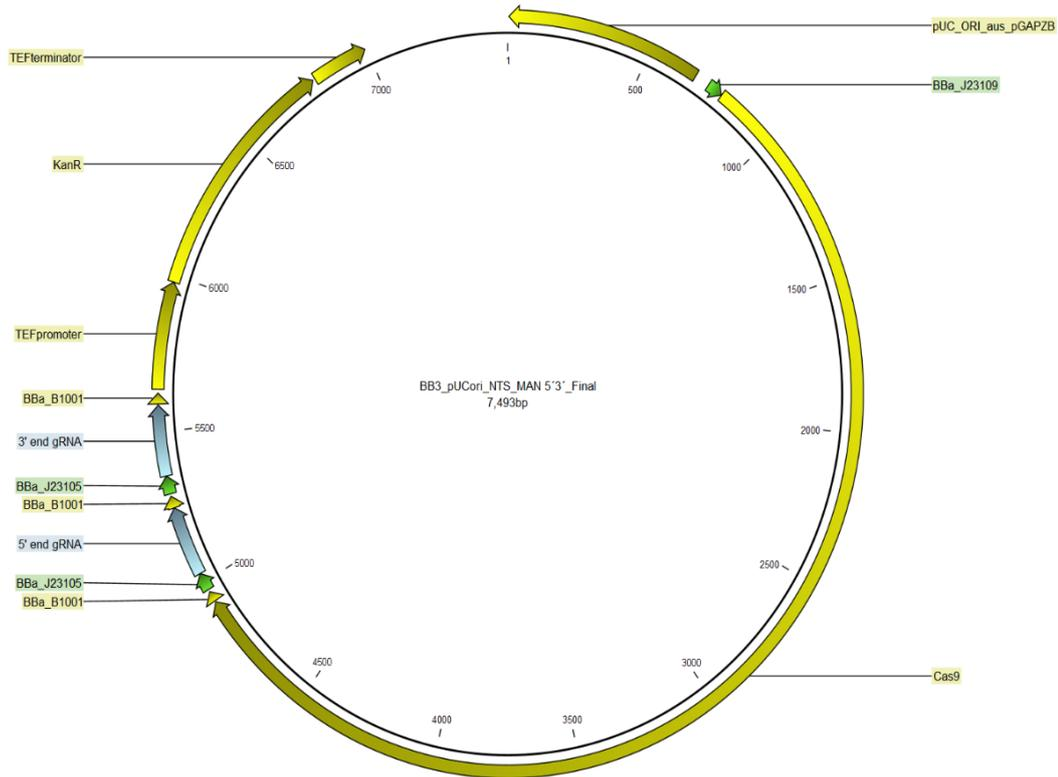
Figure 11. b) BB3\_AD\_p109\_Cas9\_p105\_MAN5'\_MAN3'\_t1001 plasmid constructed in the lab using CLC Main Workbench. BB3\_AD\_p109\_Cas9\_p105\_ptsG5'\_ptsG3'\_t1001 plasmid was constructed in the same way.
