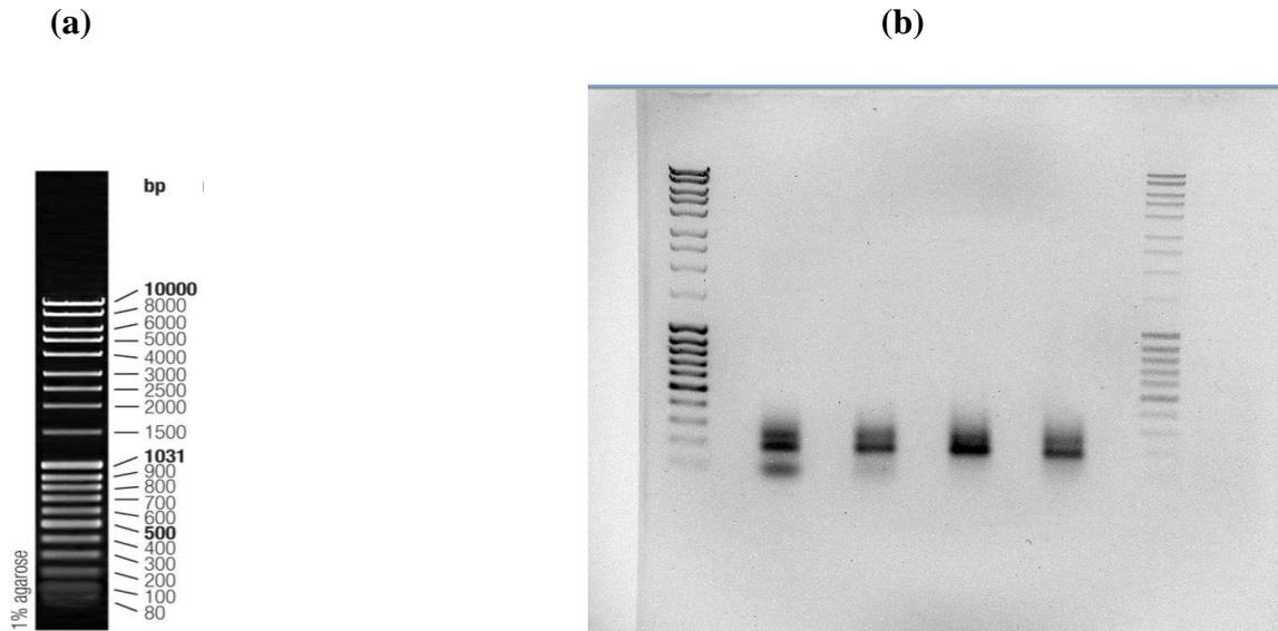
Figure 10 a) MassRuler™ DNA ladder mix (ISO 9002, 2016); b) example of gel-band 1-ladder, band 2,3,4 and 5 PCR fragments size app. 240 bp, band 6-ladder (laboratory image).
