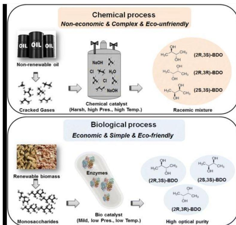
Figure 5. Comparison of chemical and biological processes for 2,3-BD production. In the chemical process, a racemic mixture of isomers is obtained from the cracked gases by a chemical catalyst, while in the biological process, microorganisms produce optically pure isomers of 2,3-BD from monosaccharides (Song et al., 2019).
