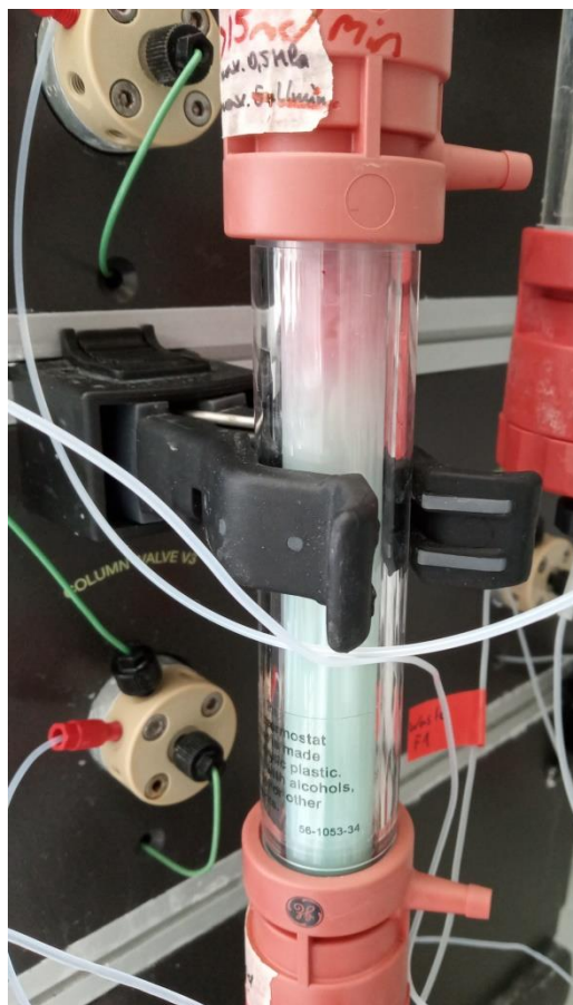
Figure 9. Binding of the cytochromes on Ni 2+ His trap column
