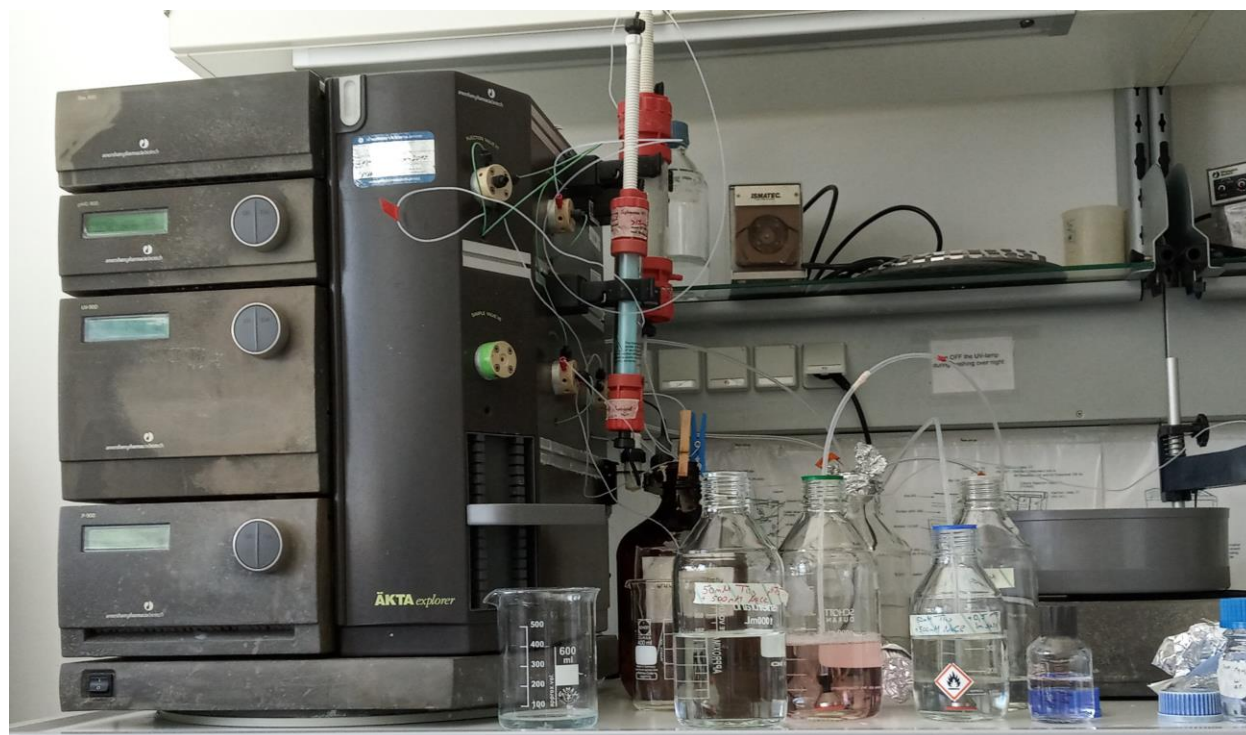
Figure 4. Cytochrome purification on Äkta Explorer (Pharmacia, Sweden) over Ni 2+ HisTrap column
