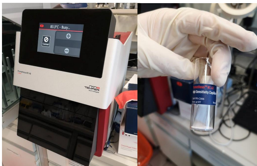
Figure 12. Prometheus NT.48 instrument + High Sensitivity Capillaries for sampling
