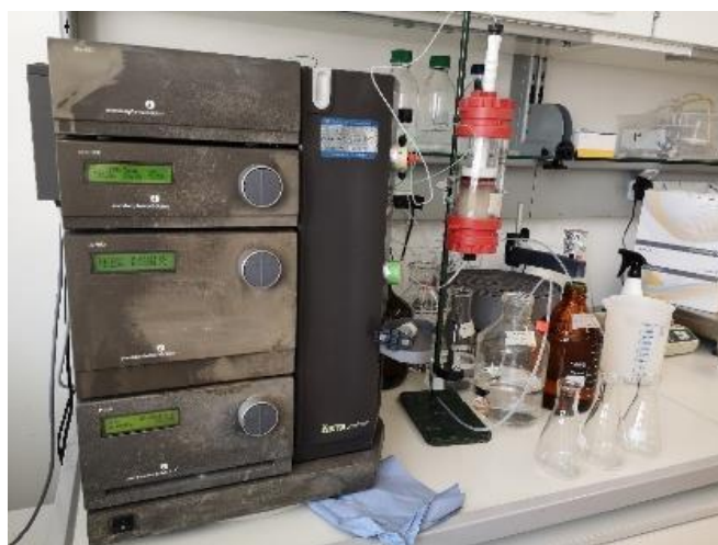
Figure 10. Äkta Explorer system with Phenyl Sepharose Fast Flow column
