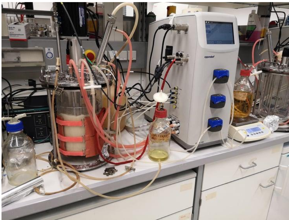
Figure 9. 5-L BioFlo fermenter with the Eppendorf BioFlo120 fermentation system as control process control system
