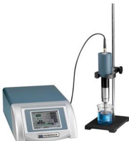
Slika 8. Ultrazvučni procesor, model S-4000, Misonix Sonicators
