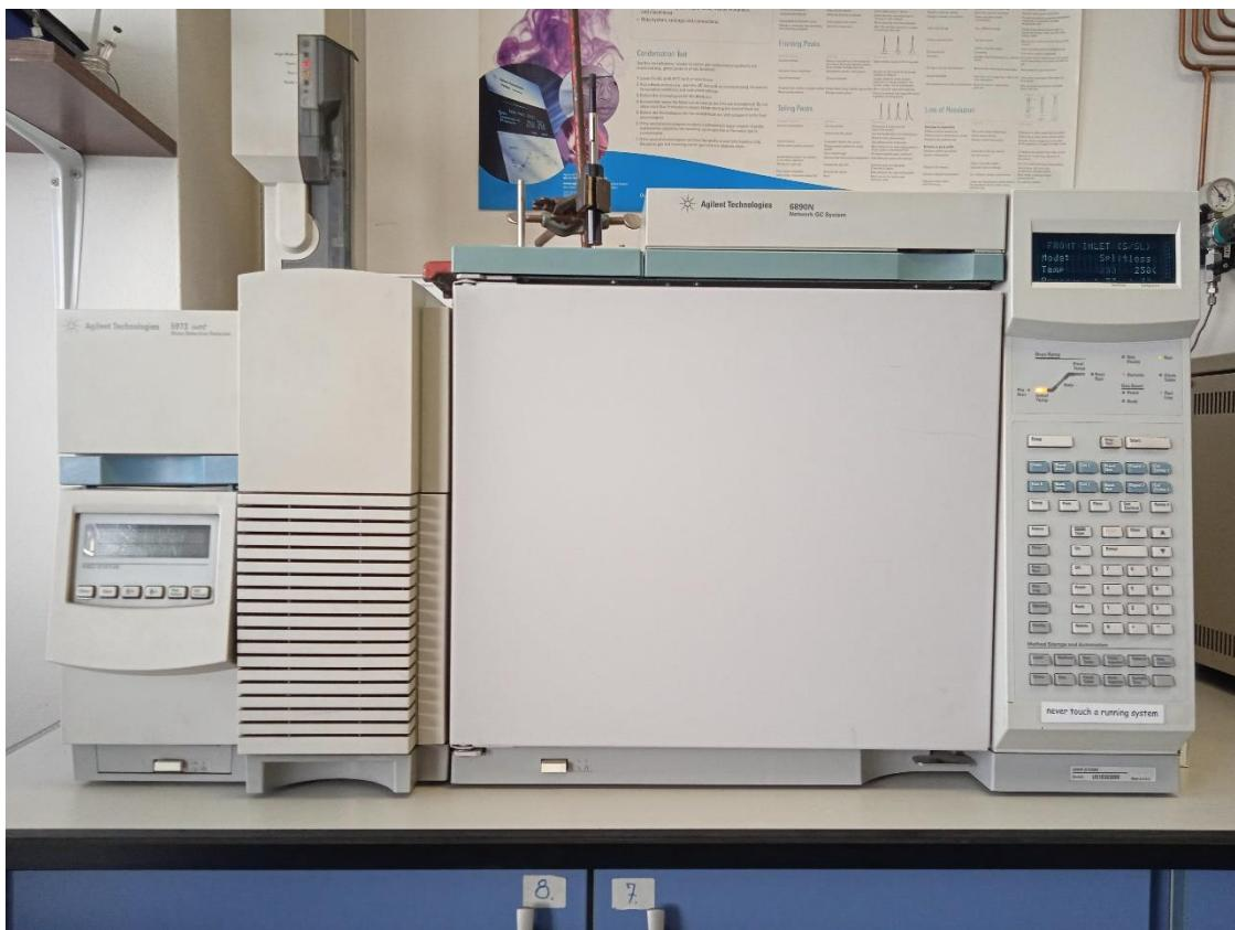
**Slika 8.** Plinski kromatograf kromatografu Agilent Technologies 6890N Network GC System
