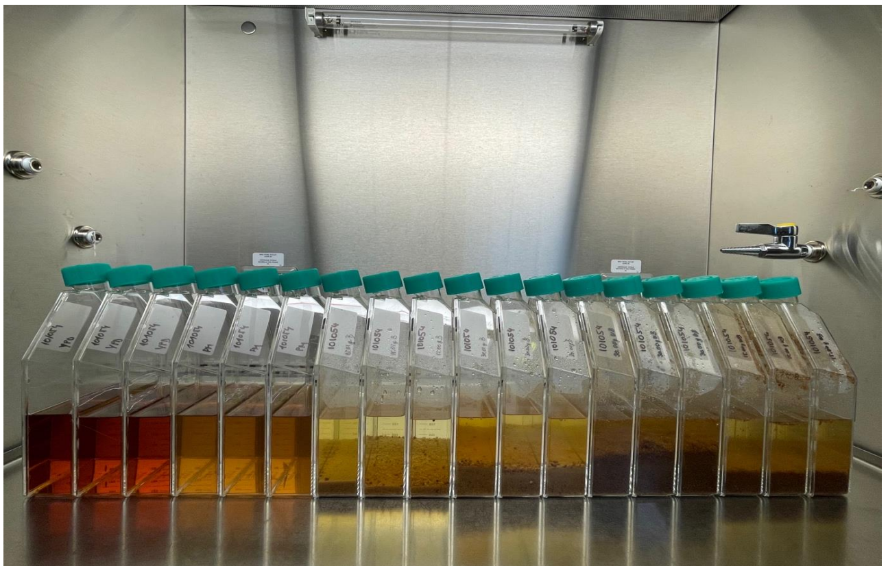
Figure 4. Media used for cultivation (from left to right; YPD, PD, bread 5 %, bread 10 %, wheat bran 10 %, wheat bran 5 %)
