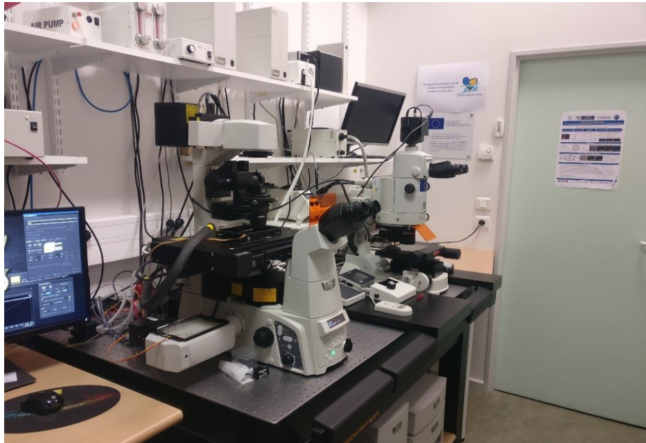
Figure 8. Microscopy equipment that was used - Nikon Eclipse Ti fluorescence inverted microscope equipped with a Photometrics EMCCD Evolve 512 camera and acquired with NIS-Elements software
