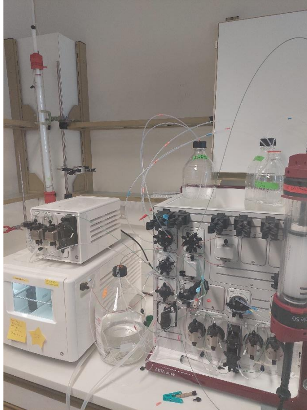
Figure 12. ÄKTA Pure Protein Purification System
